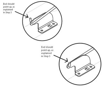
Figure 20: Left & right brackets, pointing up
