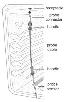
Figure 29: Using the probe
