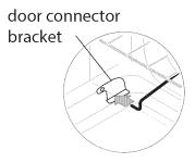
Figure 19: Connector arm/door connection
