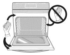
Figure 40: Clean around the oven door gasket
