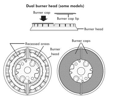
Figure 5: Dual burner head using two burner caps
