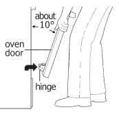
Figure 49: Holding door for removal
